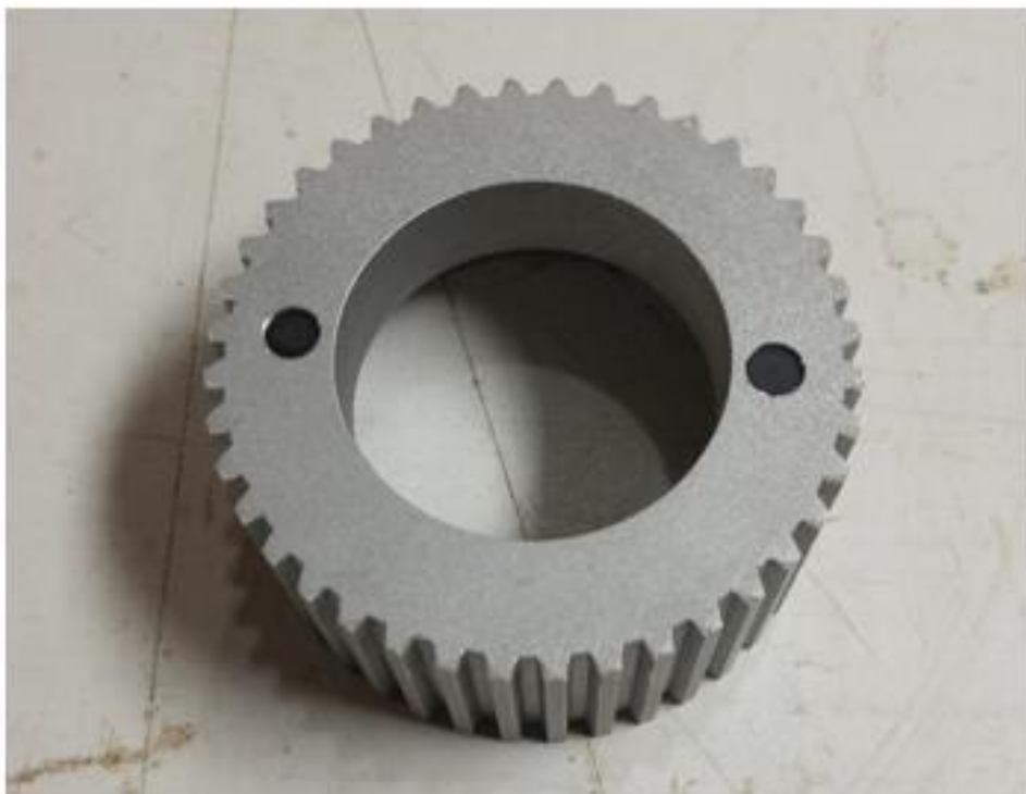
Figure 4: Completely fabricated Inner Brake (top view)
