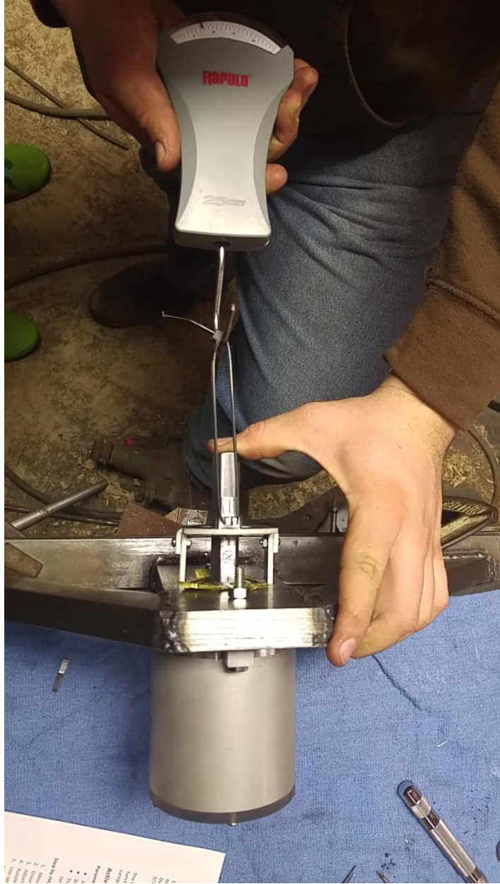
Figure 47: Actuation testing of the braking mechanism.
