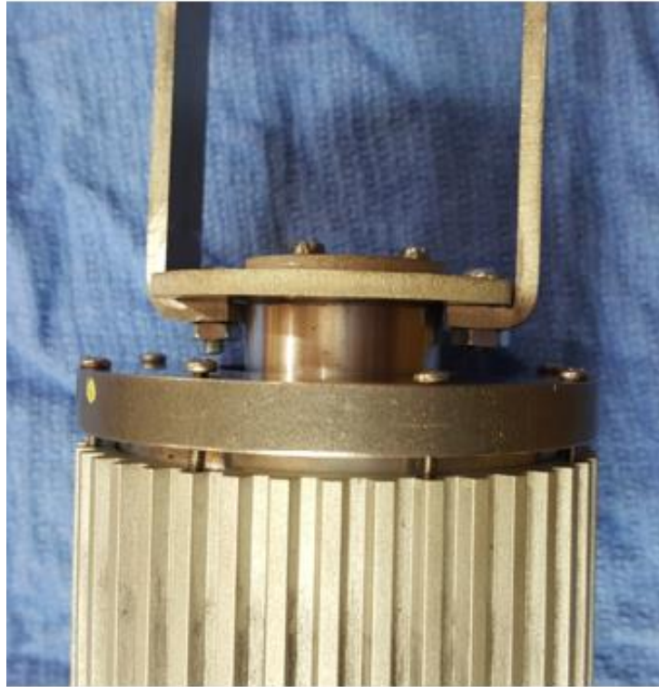
Figure 40: The Actuation Ring Links are now screwed into the Actuator Ring using 6-32 Machine Screws.
