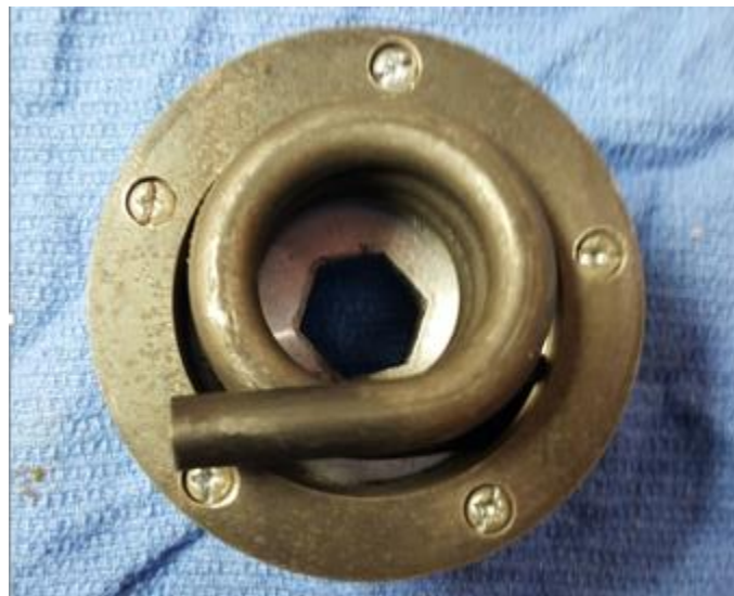
Figure 36: The Interface Plate is screwed into the Assembly Slider, over the Torsion Spring.
