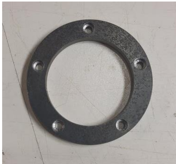
Figure 22: Friction plate Interface Ring with countersinks added.
