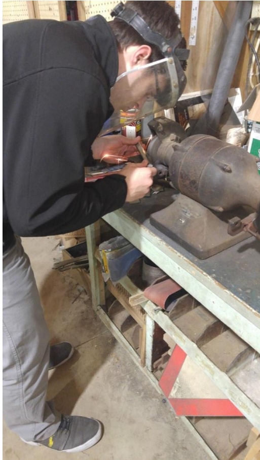
Figure 12: Grinding down faces of the Actuator Hook Rail and countersunk screws.
