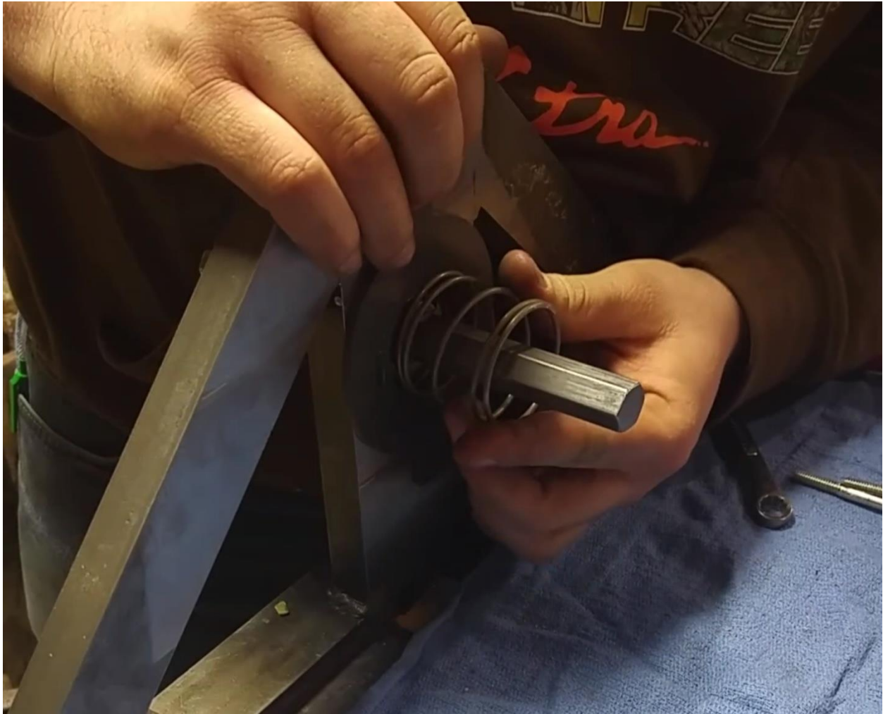
Figure 41: The Frame Side Closure Plate and Normal Force Spring are held in place.
