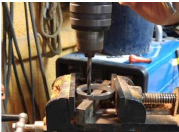
Figure 23: Drilling counter bore holes into interface ring.
