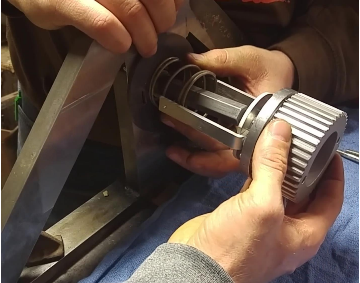
Figure 42: Sliding the Inner Brake Assembly onto the shaft.
