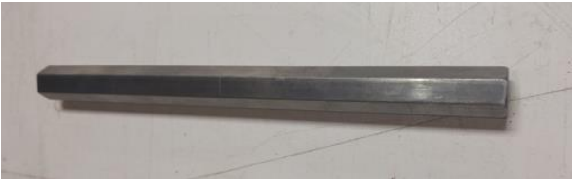
Figure 28: Hex shaft blank after being cut to length.
