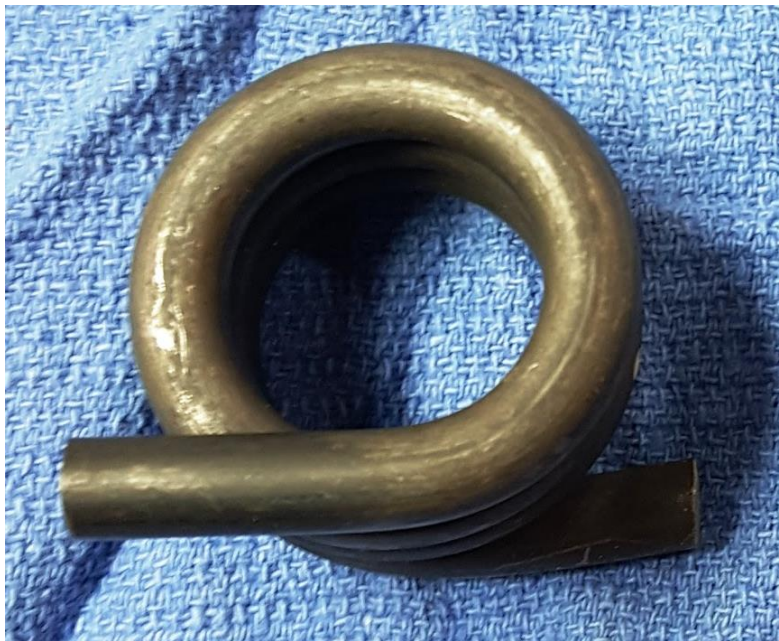
Figure 31: Picture of the Torsion Spring with shortened legs.
