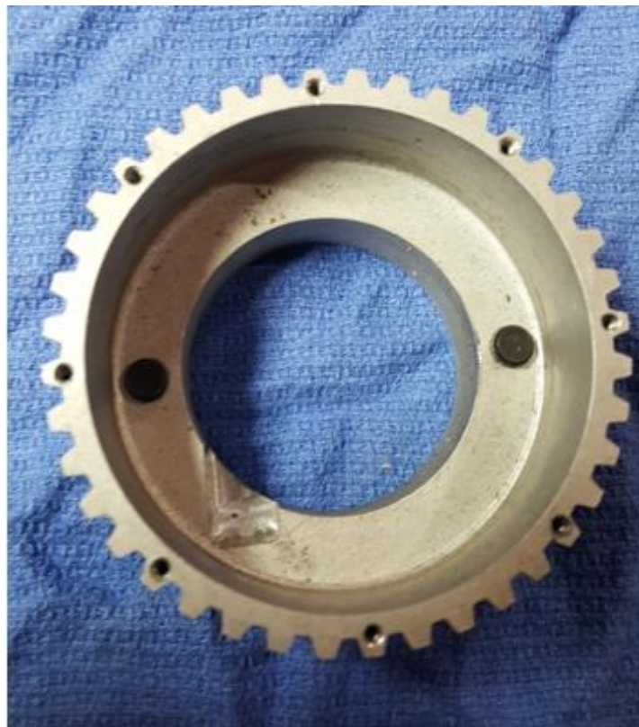
Figure 33: Dowel pins placed into the Inner Brake, ready for assembly of the Friction Plate.
