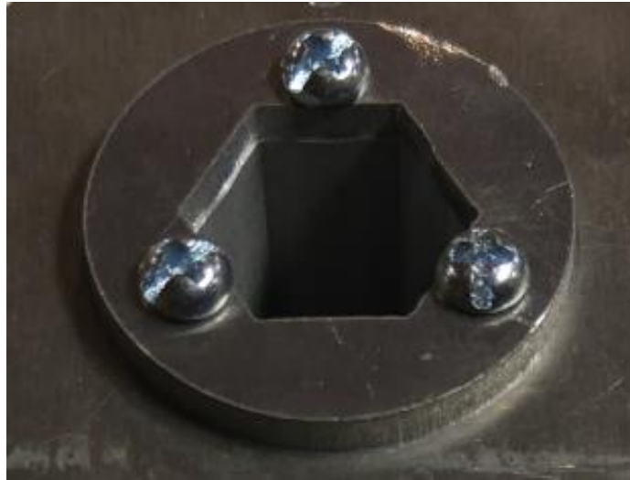
Figure 27: Finished Assembly Slider Contact Ring bolted into place.
