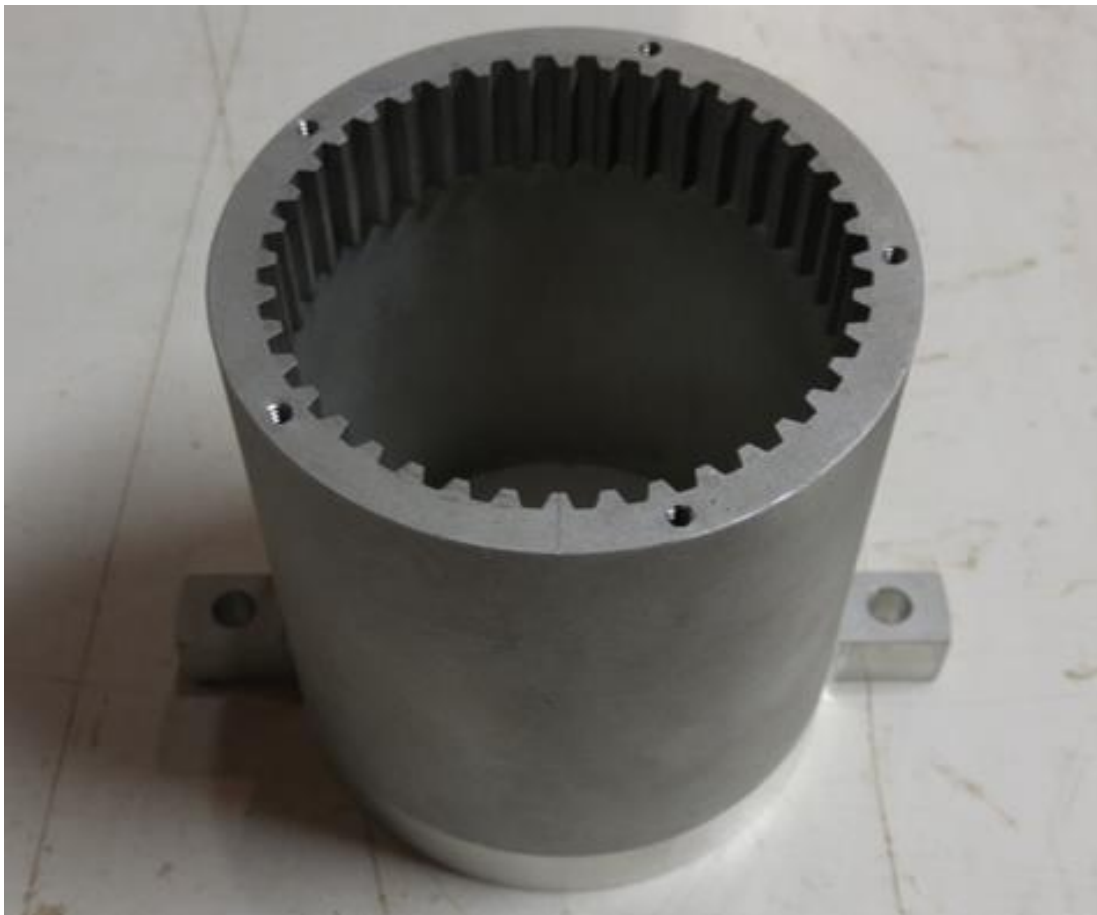
Figure 7: Completely fabricated Inner Brake (top view).
