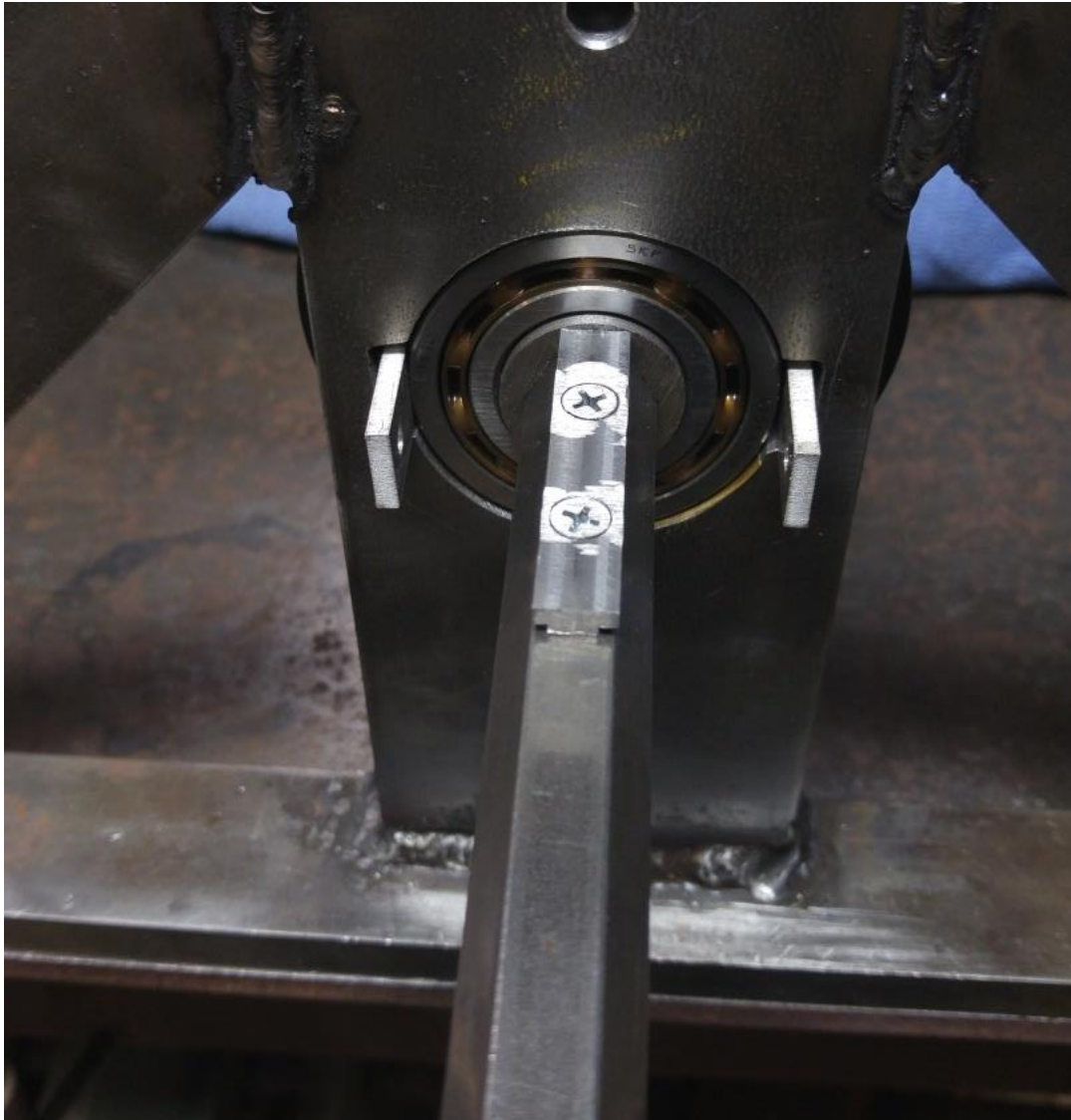
Figure 45: Actuator Hook Rail assembled into the Shaft using 6-40 Machine Screws.
