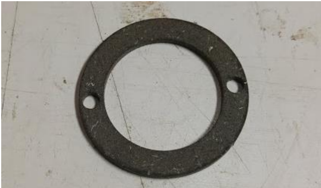
Figure 24: Friction plate with countersinks added.
