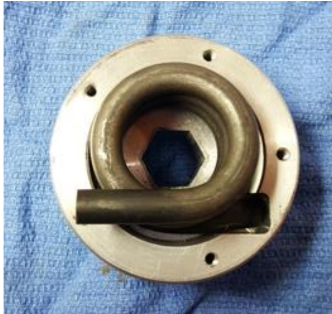
Figure 35: The Torsion Spring is placed into the Assembly Slider.
