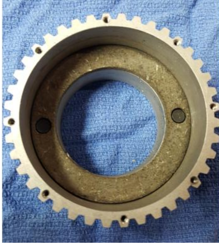
Figure 34: The Friction Plate inserted into the Inner Brake.
